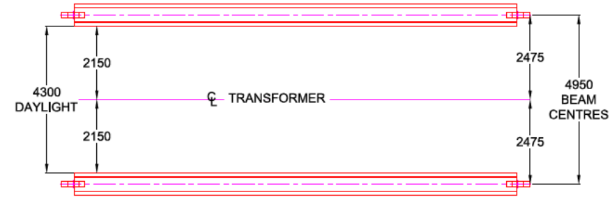
BEAM DETAILS: PLAN SCALE 1:75
